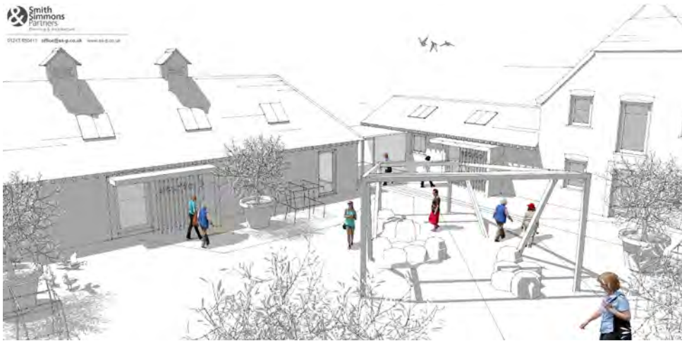
Fig 4. Introducing roof lights to gain top lit spaces
