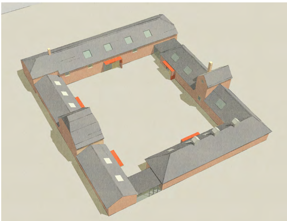
Fig 5. Suggested 'Links' between the existing building blocks to create a self-contained, enclosed courtyard
